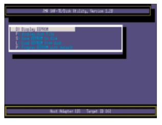
save the current firmware in the unit to a disk. *Load EEPROM from disk* will load the EEPROM file from a disk and save it in the unit as the new active firmware. The *Program EEPROM with default* command will restore factory default settings to the unit. See the section **Updating Firmware**, for specific information on using these commands and changing firmware settings.
